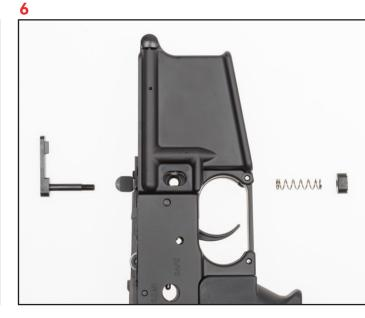
$\cdot$ Turn the magazine release button counterclockwise to remove it, then remove the related components.
