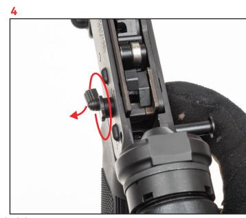
Align the fire selector lever between SEMI and AUTO. Then, push the lever shaft out from the opposite side. Finally, rotate and remove the selector lever assembly.
