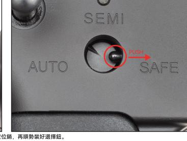
·裝回火力選擇鈕時,要指向SEMI和AUTO之間,並且需要工具輔助推開定位銷,再順勢裝好選擇鈕。 ·When reinstalling the fire selector lever, align it between SEMI and AUTO. Use a tool to depress the detent pin, then slide the lever into position.
