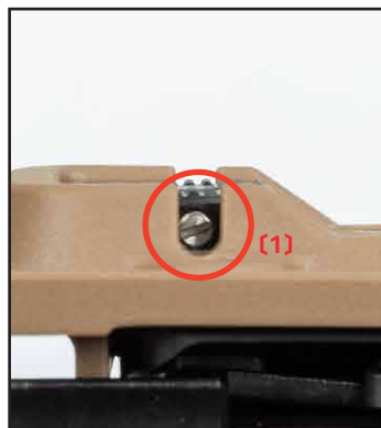
彈匣釋放鈕銷釘 (FN原廠為C型彈性銷-拆裝難度高) Magazine release button pin (FN original factory C-type elastic pin - difficult to disassemble)
